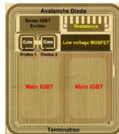
Smart Power Device with integrated sensing
